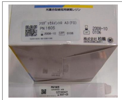
ISO/IEC 18004 QR码中含有HIBC代码 HIBC carried by QR Code ISO/IEC 18004
